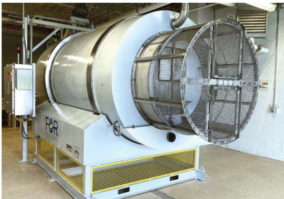
PLC panel, discharge end of vessel with attached screener.
