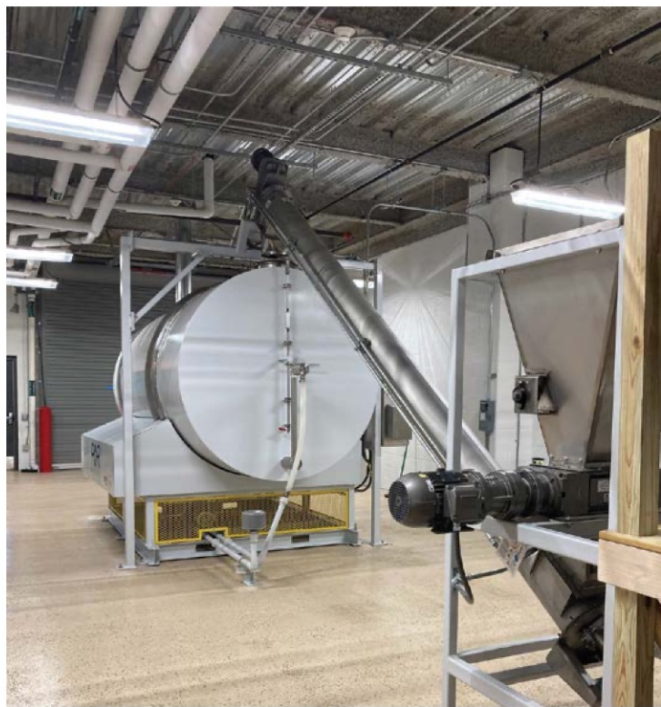
Loading hopper, shredder, screw conveyor, and input end of vessel. Images courtesy of FOR Solutions.
